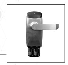
Insert the Battery Pack in the Inside Cover using one (1) flathead M4x12 hex screw. After the screw is fully tightened, loosen the screw by one full turn.
