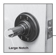
The large notch on the Outside Shank should face away from the edge of the door.
